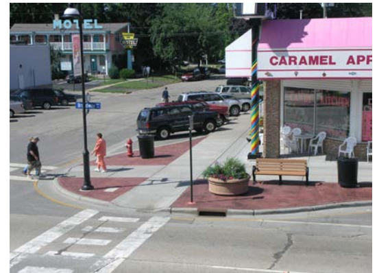
Figure 2. Curb Extension at a Street Intersection
